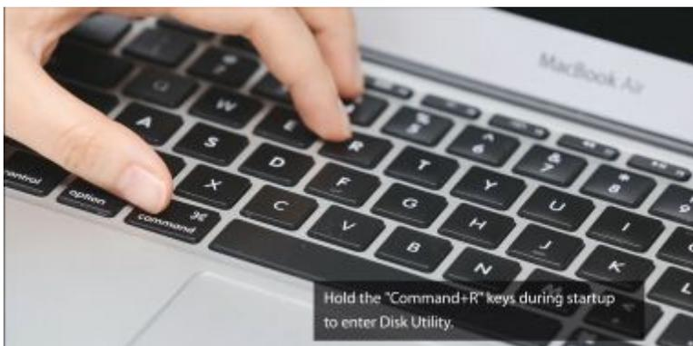
Hold the "Command+R" keys during startup to enter Disk Utility.
